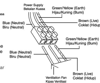
Connect the power cord to the power supply according to the diagram attached.
