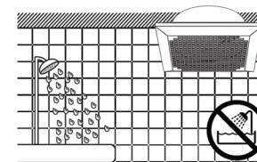
Do not install the ventilation fan in high humidity and wet area.
