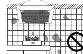
Do not install the ventilation fan over cooking area and area with extreme heat.
