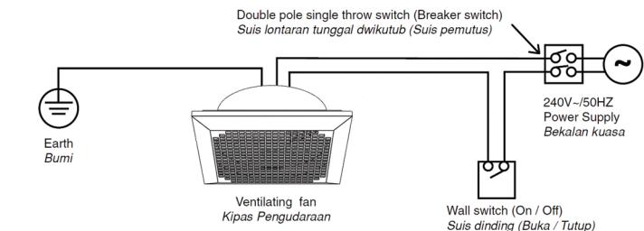
Only direct connection to wall switch is allowed. Please refer to figure shown above. Eco Breeze will not be responsible for any unwanted incident caused by any alteration in installation.
