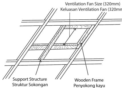
Fix a wooden frame to the ceiling support structure and make sure that the support structure on the ceiling is stable. Make sure that the wooden frame's opening size matches the frame size of the ventilating fan (320mm).
