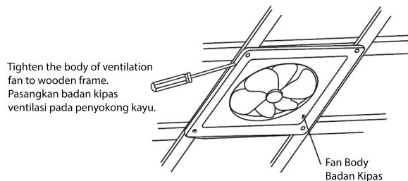
Install the set to the wooden frame using the screws provided. Make sure that the set is fully secured before operating.
